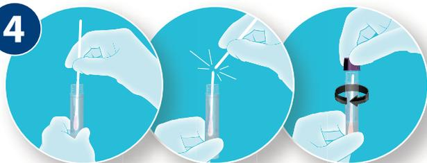
Place swab into the viral transport medium and break (snap) off swab at the indicator line. Replace cap and screw on securely.
